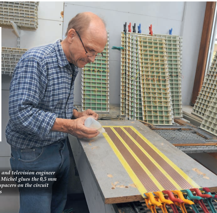
No undesired vibrations: All the connections on the stators are newly glued.
