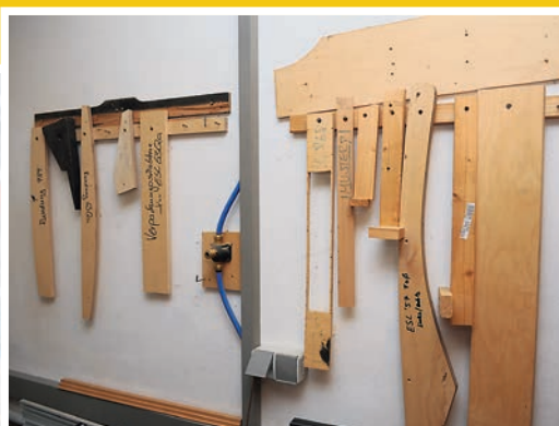
The storeroom contains templates for all the wooden parts of the electrostatics
