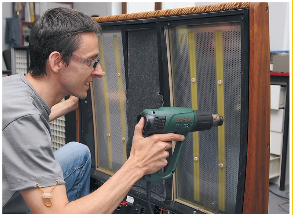
Weber seals the rear with a transparent foil to protect the delicate Mylar film and stators from dust – blow-dried crease-free, of course!
