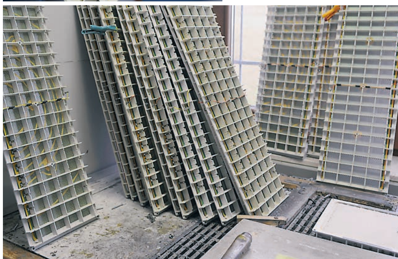
Dry dock: Before the next production step the special glue on the freshly glued plastic stators must thoroughly harden. The slightest carelessness during the preparatory work can be audible in the final product...
