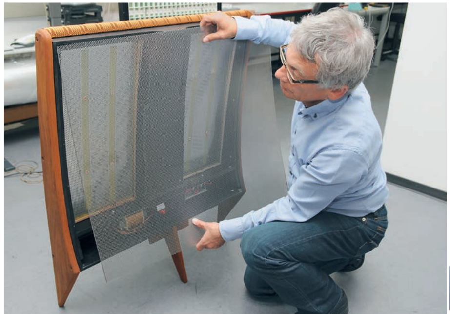
Just to make sure: The rear of the soundboard must also be closed with a thin metal grid
